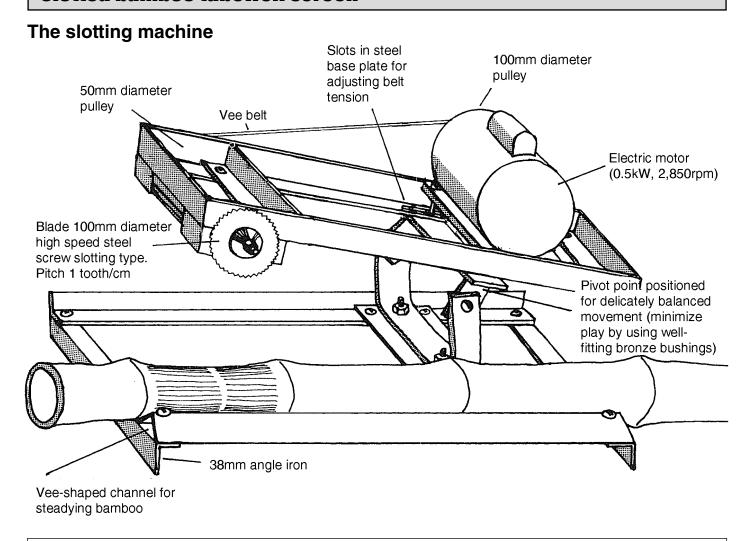
Note: For clarity, this drawing shows the machine without safety guards on belt and blade. These are essential for safe operation.
