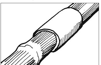
Bamboo to GI: cut threads in the end of the bamboo filter and use a threaded GI socket.
