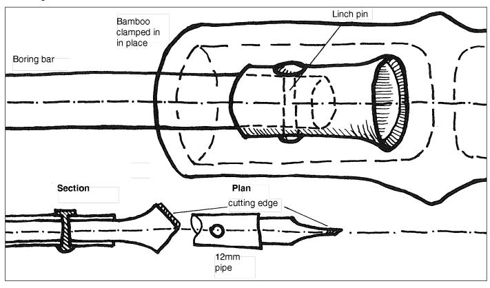
To make the bit illustrated (top), bell out the end of a short length of steel pipe to increase its diameter, and sharpen the edge. Slide the 12.5mm diameter steel pipe inside as a boring bar. Drill a small hole through the assembly and drive a nail through it as a linchpin.
