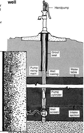
A good screen should hold back sand particles after the initial development of the well and let water flow in freely at the same time. It should be strong enough to withstand handling during installation. It should also be resistant to corrosion.
